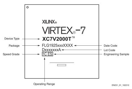
Figure 1: Example Device Top Mark
